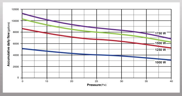
Acummulated daily flow vs. pressure for Florida at different solar PV capacity.
