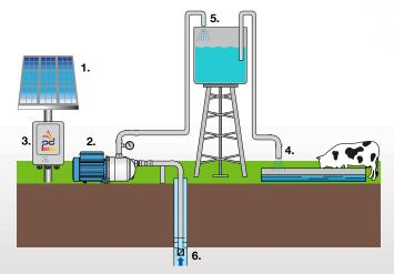
PD Solar designs your system based on the most cost effective turnkey solar array to power the water pump stations.
